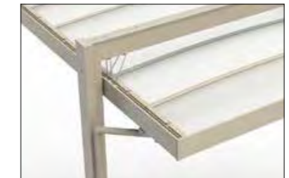
Roof suspended from beams
