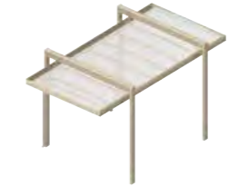
Roof suspended from beams
